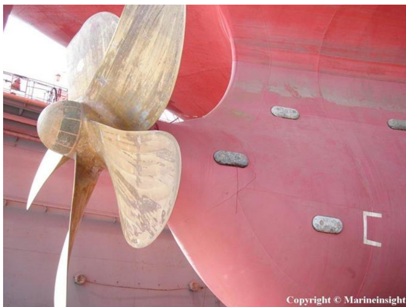
Figure 2 – Placement of protectors on the ship's hull
