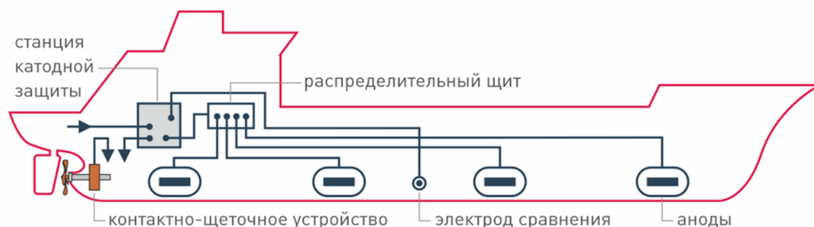
Figure 1 – Scheme of cathodic protection of ships
